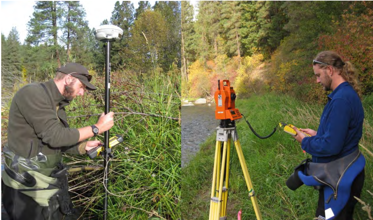
Figure 4. Survey grade RTK GPS (left) and Total Station used to collect DEM data of the Icicle Creek historical Channel Study Site.
